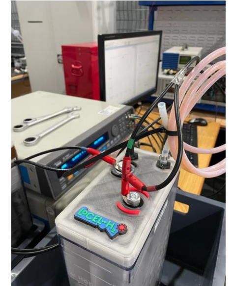
EIS initial frequency of 9400 Hz and final frequency of 0.1 Hz
