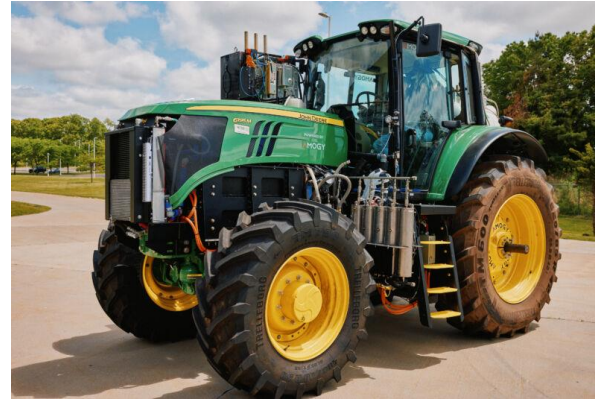
Amogy's "ammonia to power" zero-emissions tractor.
